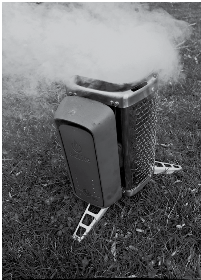
This is what happens after too many pellets or twigs are added too quickly.
