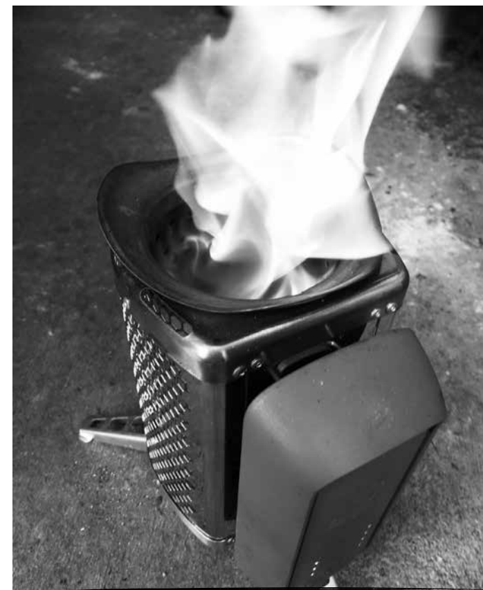
Wood fuel is releasing gases that are drawn down and into the side wall chamber. As these gases re-enter the burn chamber through top holes, they ignite without causing any smoke.
